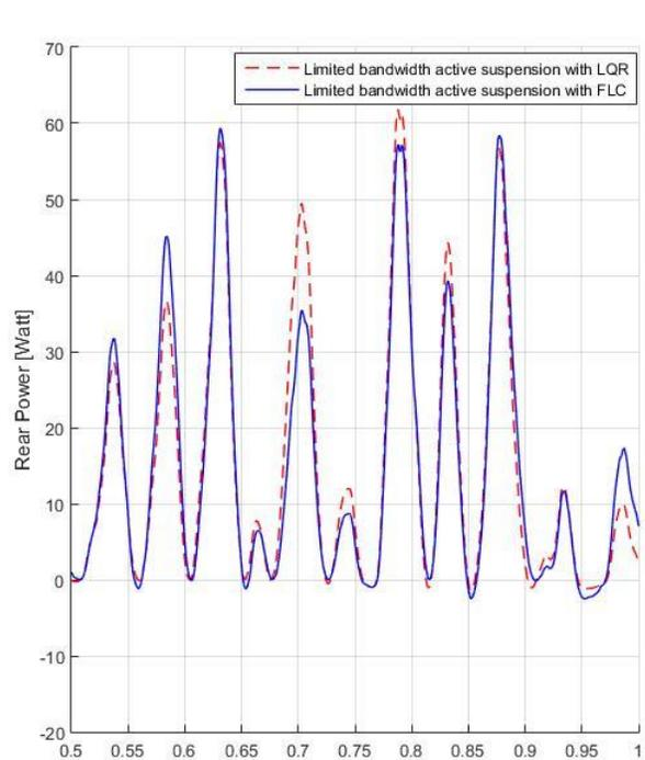
Fig. 6 Comparison between LBA suspension with LQR and FLC at front and rear in terms of power demand
