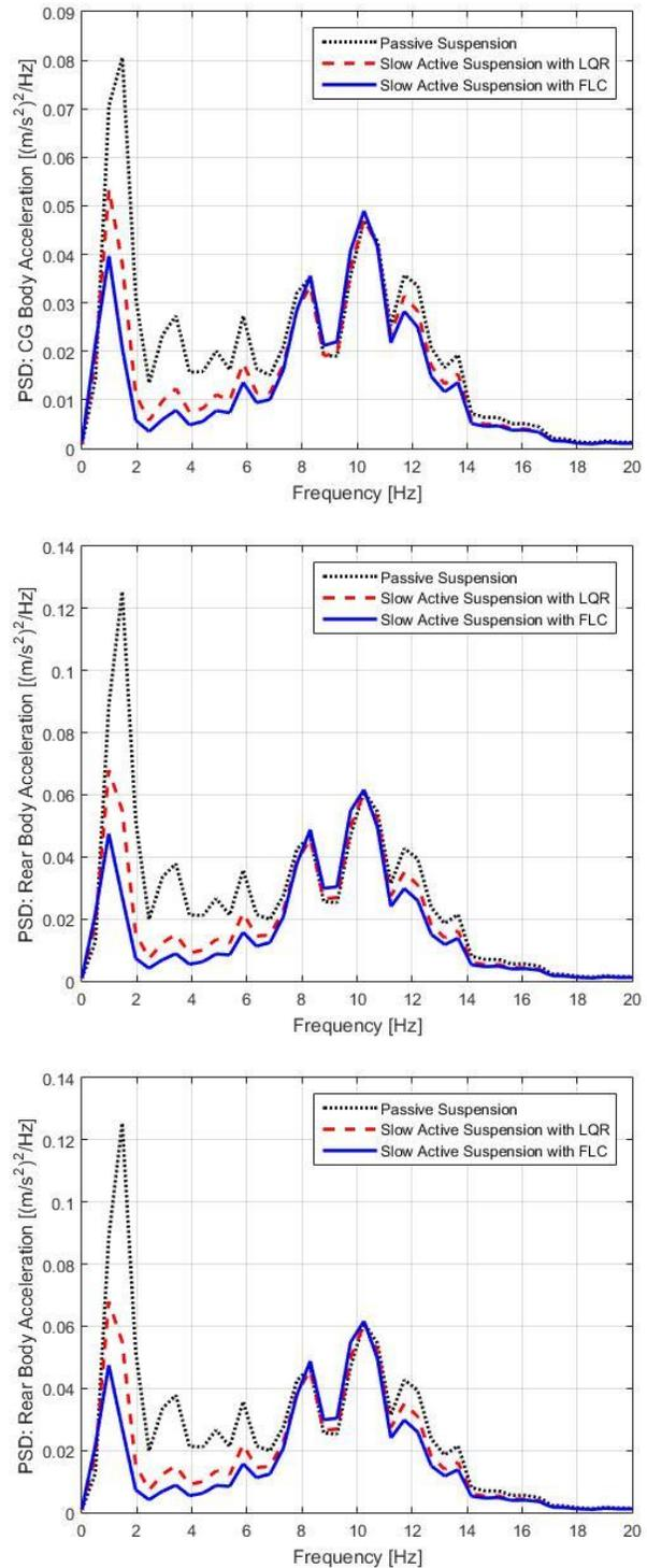
Fig. 2. Power spectral density of body C.G bounce, pitch accelerations and rear body acceleration for passive and LBA suspension with LQR and FLC using road input (class B)
