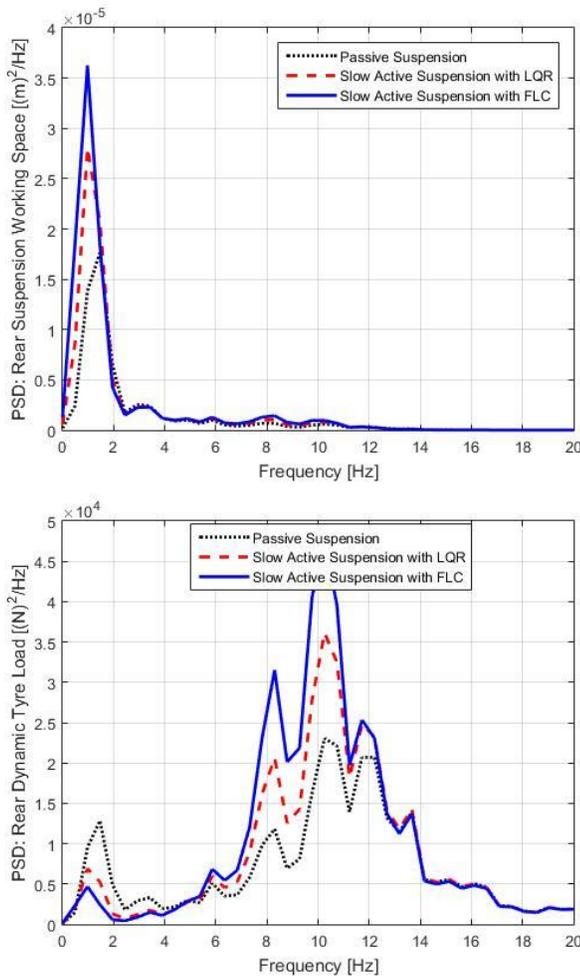
Fig. 3. Power spectral density of rear SWS and DTL for passive and LBA suspension with LQR and FLC using road input (class B)
