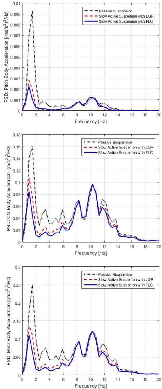
Fig. 4. Power spectral density of body C.G bounce, pitch accelerations and rear body acceleration for passive and LBA suspension with LQR and FLC using road input (class B)
