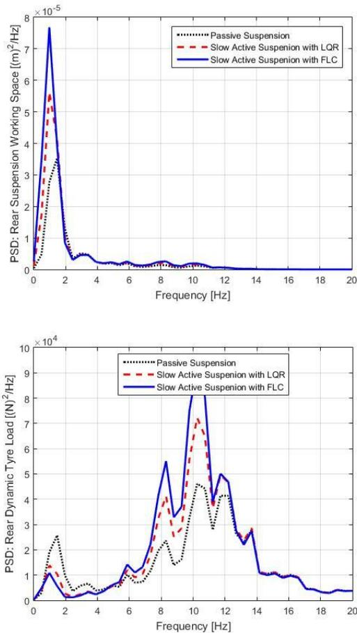
Fig. 5. Power spectral density of rear SWS and DTL for passive and LBA suspension with LQR and FLC using road input (class C)
